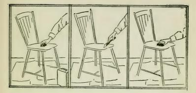
These sketches suggest ways of holding implements for removing old finish and preparing new furniture. Note the scraper and rubbing felt.
